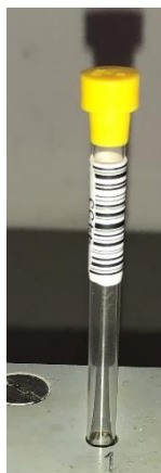
Figure 2: Barcode placed on NMR tube.
