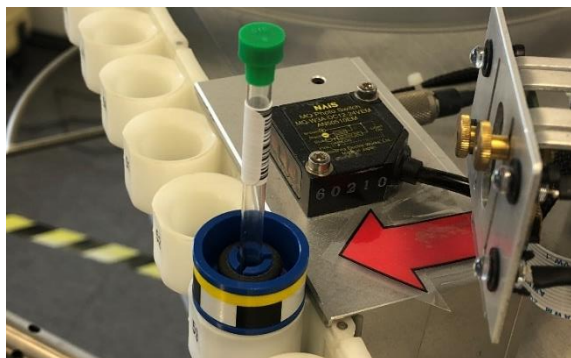
Figure 4: Marked position where to place a new sample. Barcodes adjusted to the barcode scanner.
